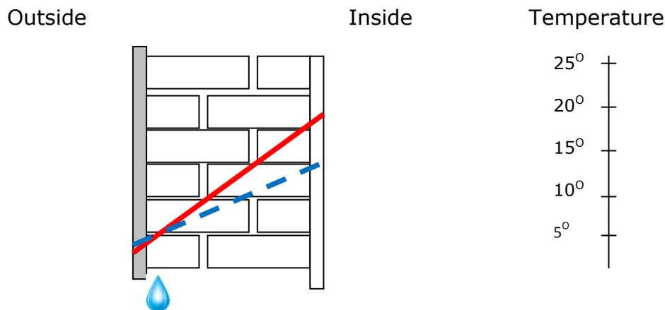
The other external treatment is to apply an external layer of insulation. Again, it has been common to use an impermeable material. This, like the hard render coating will trap moisture within the brickwork and raise the dew-point temperature (the dotted blue line). When the two lines meet, water will condense.
