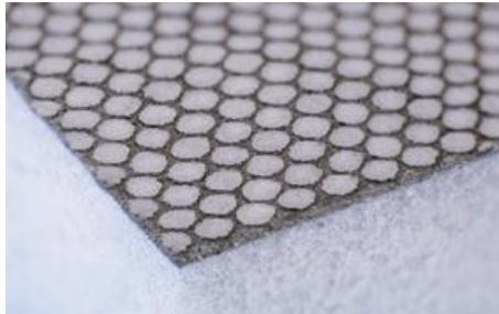
Dry-lining insulation with Marmox Multiboard simplifies this operation because it is both an insulation board and because it is waterproof, it acts as a vapour control barrier. Because Marmox is a moisture barrier, the water vapour inside the house cannot get into the wall to start with so there is therefore a lower vapour pressure so less moisture to condense.
