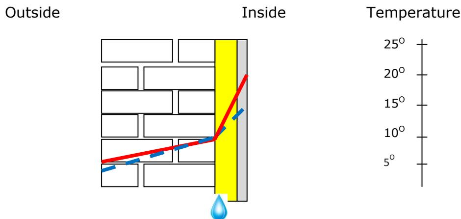
One solution to protect the insulation is to include a VAPOUR BARRIER behind the insulated plasterboard which is generally a single continuous sheet of polythene. This also poses problems since if the barrier become broken, ripped or acquires just the smallest puncture marks, water will accumulate there and there will be a bloom of localised damage.
