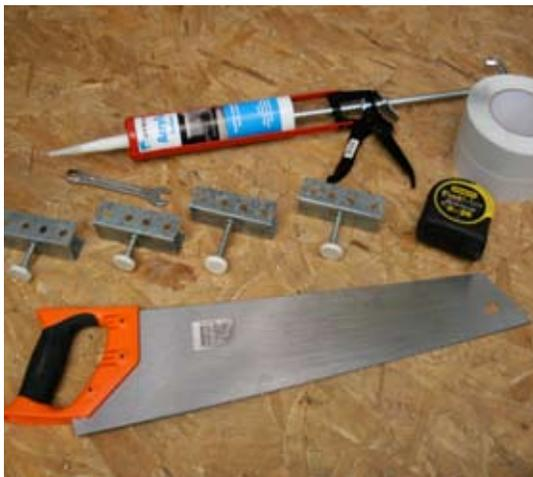
**1** Check you have all tools needed. Marmox Bath Panels come in two sheets, 1800mm x 600mm x 30mm and 800mm x 600mm x 30mm.
