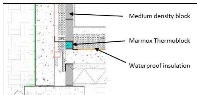
**Specification to eliminate or reduce thermal bridge at the base of an external wall with the basement floor**
