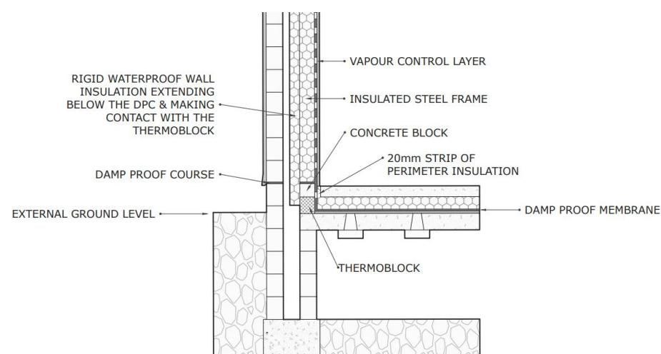
**Specification to eliminate or reduce thermal bridge at the base of a steel frame wall with a suspended OR ground bearing slab**
