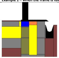
The  $\psi$  value of this particular junction has been calculated and published by the BRE in their Certified Thermal Details Scheme giving a  $\psi$  value of 0.058W/mK
